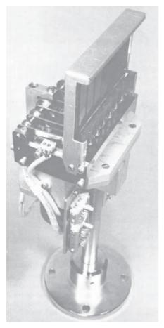
Figure 6: Jalousie monochromator with seven graphite crystals
