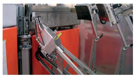
Figure 12: Analyzer and detector banks of the backscattering spectrometer MARS at SINQ
