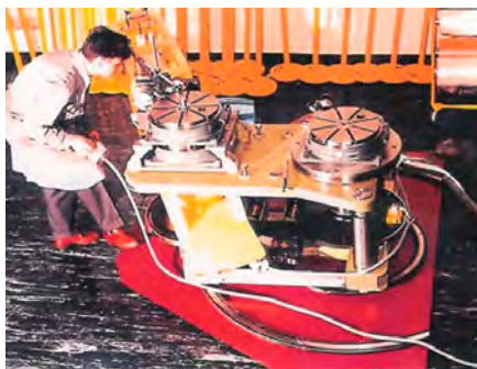
Figure 2: Main mechanical parts of the first neutron diffractometer at reactor SAPHIR, supervised by the mechanics expert M. Koch.
