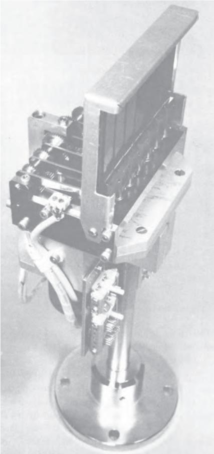
**Figure 6:** Jalousie monochromator with seven graphite crystals
