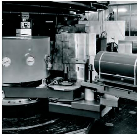
**Figure 2:** Three-axis spectrometer at Diorit. The monochromator is built on top of a rotating anti-aircraft-gun carriage.
