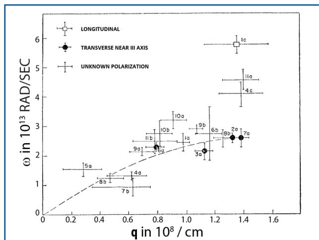
Fig. 2 The relation between the phonon frequency,  $\omega$  ( $10^{13}$  radians/sec) and the phonon wavevector,  $q$  ( $10^8 \text{ cm}^{-1}$ ), near the [111] direction in aluminium (Al). Positively identified transverse (TA) and longitudinal (LA) modes are indicated by solid and open circles. Phonons of unknown polarization are indicated by dots. The dashed curve is a sine curve whose initial slope corresponds to a velocity of sound of 3080 m/s for Al.
