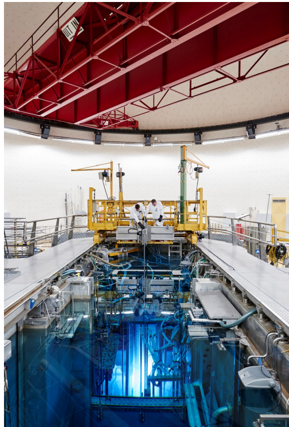
Figure 21: Operators manipulating isotope production equipment in the HFR pool.
