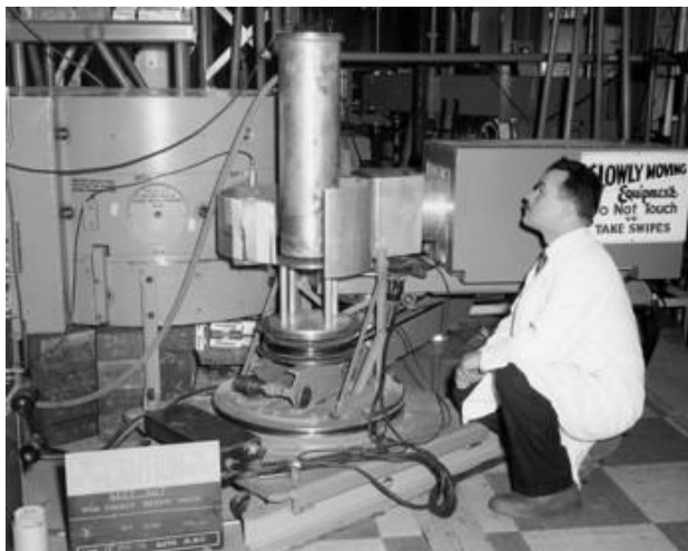
B.N. Brockhouse with the first version of his triple-axis spectrometer at the NRU reactor (November 1958 - July 1959). The cryostat carrying the specimen could be moved at half the scattering angle by a system of steel belts originally developed in 1947.
