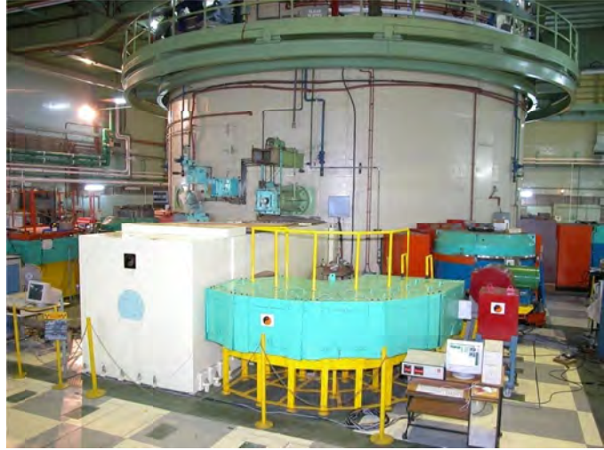
Fig. 25. Diffractometer based on multi-monochromator layout. White monochromator shield and green detector shield are seen in the photograph at Dhruva
