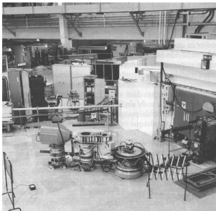
Figure 3.2 Photograph of the original IN2 triple axis spectrometer showing the large sample table, analyser, and detector after the double monochromator in the shielding to the right.
