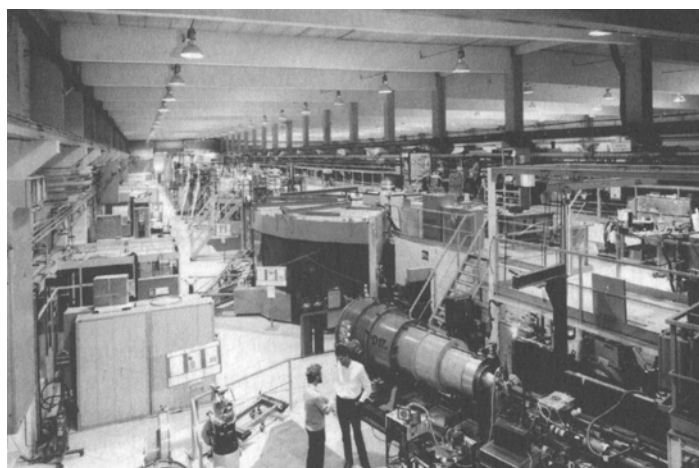
Figure 5.9 A view of a part of the guide hall with some of the instruments installed on the cold guides. In the centre is the shielding for the detectors of the time of flight spectrometer described above (figure 3.4) The instruments are painted in vivid colours. This was started in 1972 to create a more cheerful atmosphere for the visitors.
