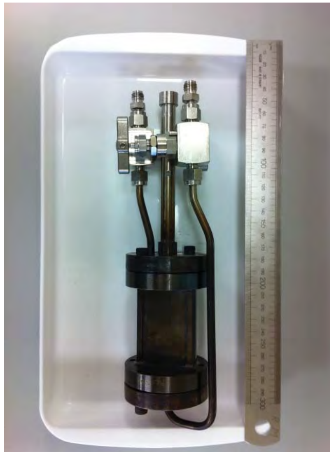
Fig.13. INS cell designed to carry out high-temperature and high-pressure (600°C, 20 bar) reactions. The cell body is made of Inconel™. Similar designs are used for less severe operation: 316 stainless steel (300°C, 5 bar), aluminium (100°C, 1 bar) and TiZr (100°C, 1 bar). The background scattering from the cell decreases in the order given. TiZr is not suitable for use with hydrogen due to rapid embrittlement above ~50°C (21)
