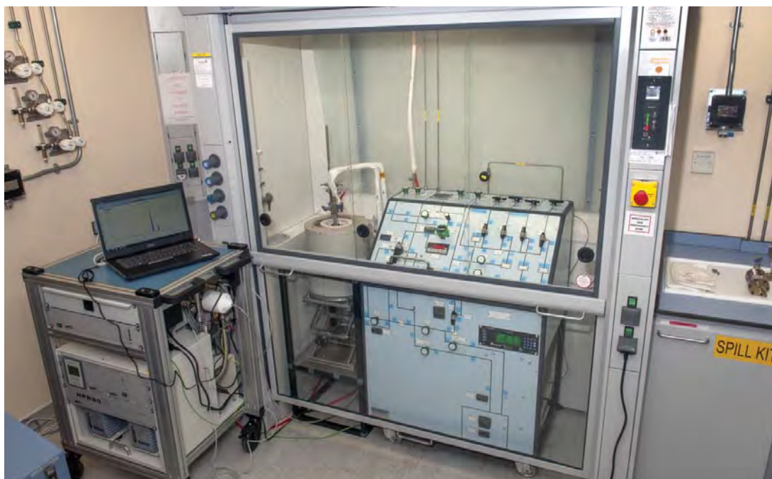
Fig. 12. A photograph of the gas handling apparatus (blue panel), that is housed within a walk-in fume cupboard. The furnace is located to the left hand side of the gas panel and is mounted on a heavy-duty lab-jack. A cell is in the furnace, which is connected to the gas panel by heated lines that terminate in high-temperature valves, which may be used to isolate the cell. The reaction may be followed by online mass spectrometry using the Hiden RGA on the trolley at the left of the picture. Toxic gas ( H_2 or CO ) monitors (black boxes on the walls on the extreme left and right of the picture) are integral to automatic safety shutdown safeguards. A more complete description is given elsewhere (21)
