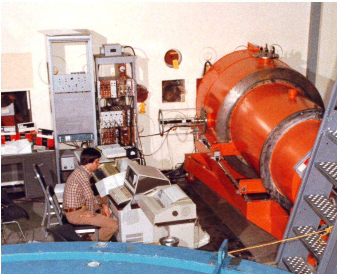
The original 8 meter SANS instrument commissioned in 1981, taking almost every inch of space available in the NBSR confinement building. Seated at the instrument station is Charlie Glinka, the leader in the development of all the NIST SANS facilities.
