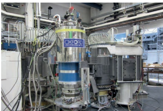
| The spectrometer FLEXX at BER II of HZB for measurements of structural and magnetic excitations in matter. This instrument combines a classical triple-axis spectrometer with neutron spin-echo technique, which boosts its resolution by more than one order of magnitude [10a]. Spin-echo techniques are also extensively used in nuclear magnetic resonance (Copyright Klaus Habicht, HZB).
