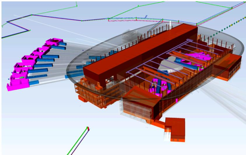
Computer model of the Target Station and Instrument Halls at ESS. The instrument sample environments and detectors are located within the pink areas. IMAGE: ESS
