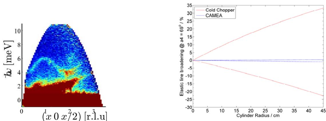
Figure 12: Examples of direct time-of-flight spectroscopy data polluted by sample surroundings. Left: CNCS, LNS data on  $\text{CoCl}_2 \cdot \text{D}_2\text{O}$  taken with the 40.5 cm radius 16 T magnet Fat Sam. No inelastic data below 3.5 meV can be seen directly due to the noise from the magnet. Right: The maximal region that can be covered by neutrons performing two scatterings in a cylinder of a given radius as seen from the centre of the CAMEA detector.
