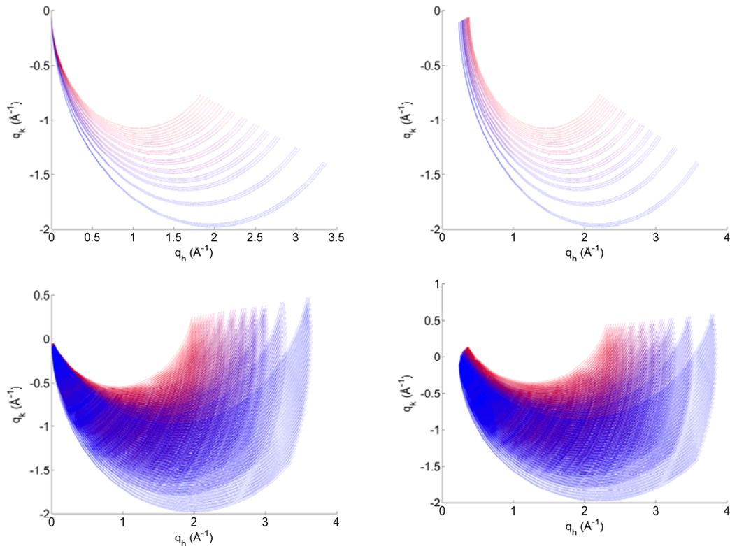
Figure 9: Schematic diagram of constant  $\hbar\omega$  coverage with  $\hbar\omega = 0$  at left and  $\hbar\omega = 2$  meV at right. On the top a single scan step is shown and below 31 steps of  $1^\circ$ . The number of analysers, that are active for a given energy transfer will depend on the chosen incoming wavelength band.
